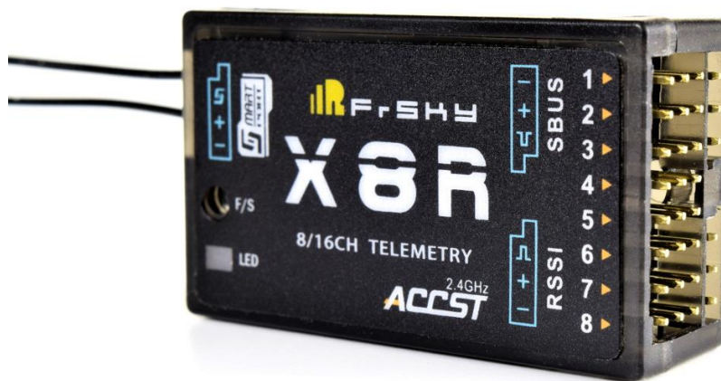
Figure 4. FrSky X8R Receiver. The external pins for all 8 channels are easily accessible.
